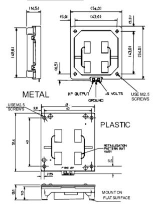
NOTES Detection range is dependent on size and reflectivity of target and S/N ratio
